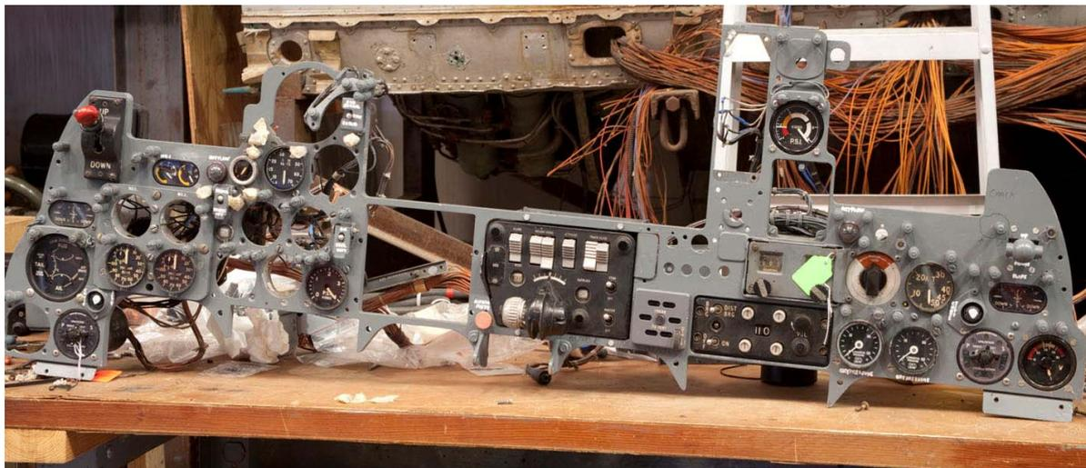
There is still a little more to do with the main instrument panel and a number of incomplete electrical and structural 'fixes' to complete in the cockpit before the panel can go in. It is hoped this will now come to fruition in the spring of 2011. It is also the view that while out of the cockpit it is less susceptible to damage while the engineers and electricians are regularly climbing in and out of the cockpit. Great progress though!
