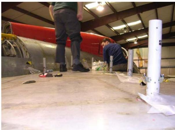
While all this was going on Milton and Rod busied themselves with the removal and testing of the fuel capacitance units from both wings. A very visual process which involves wiring the units together to mirror their set up in the wing and then submerging them in fuel to simulate 'full' and then removal from the fuel to simulate 'empty' while measuring their capacitance on a test rig.
