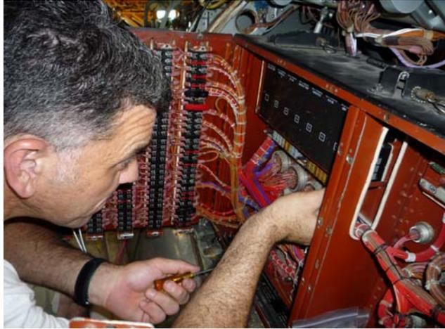
Following their departure Rod was joined, a week later, by Nick Woodhouse & Andrew Brodie. In the interim Rod continued working up a detailed electrical survey of XS422, front to back, which will form the basis of electrical work on the aircraft from here on in. This highlights missing items or unfinished areas of work, plus any snags.
