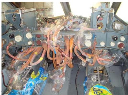
The progress made and the goals achieved mark the visit as a great success. In particular, the identification, inspection & cleaning of connectors for the main instrument panel achieved an 80% success rate on first pass. Later in the trip the remaining 20% were also wrapped up. All the connectors were then bagged up with their idents ready for John Watson & Dave Dunn to continue progress in November.
