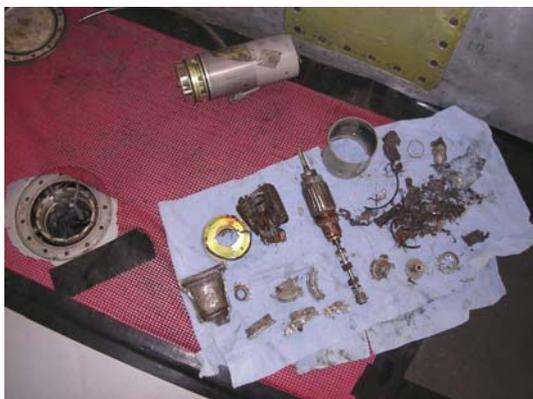
Yates to remove the remains of the pump. Failure would have meant replacing the whole leading edge tank with the spare at Bruntingthorpe, a delay and costly step backwards.
