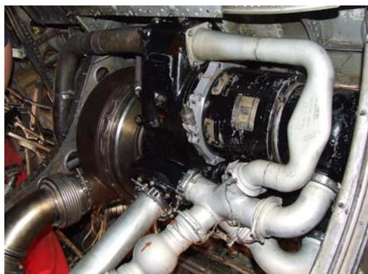
A further unexpected bonus was that with the donation of the use of an Air Start Trolley from Stennis Airport Authorities, the ATGB was run up inside the aircraft for the first time in 14 years and ran for 2 or 3 minutes no problems. An amazing achievement as the gearbox had travelled half-way around the world for its restoration.
