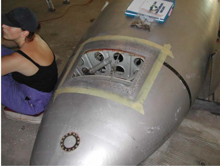
Jason Skinner who is an Avon specialist concentrated on the power plants and spent many hours checking them over and applying new inhibitor as specified in the maintenance manuals. Jason then went through the throttle runs making a list of required spares and checking routing and connections. AALO believe that all the required items are in stock and Jason will be working up the spares package needed for the US team to finish this vital area of the restoration.
