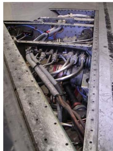
Additionally, terminal blocks in the cockpit floor were identified, marked, photographed and then removed, as well as the same blocks from ZF597's cockpit, which is also housed at Stennis. Generally the blocks were found to be in good condition although the identifying took a while as many were faded. All the blocks have been returned to the UK for restoration or replacement and John will hopefully be back at Stennis in November to secure them back in the cockpit floor.
