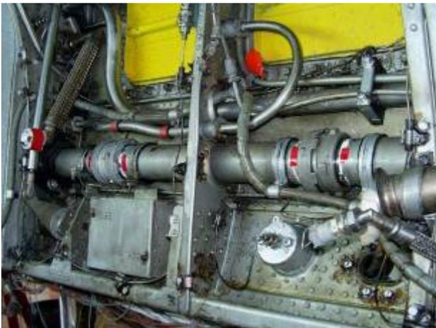
*FRS Couplings (identified with red tape) in No 1 Engine Bay ready for X-Ray shots*
