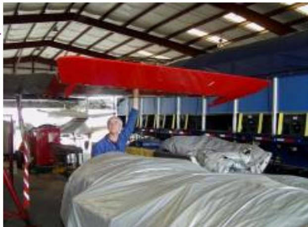
*Rear Centre Section Heat Shield is being fitted by Dave*
