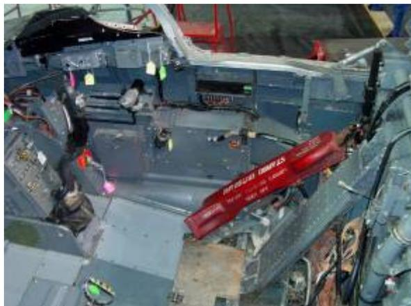
Myself, Geoff and Dave Yates started work on the 20th Mar our prime objectives being the preparation of the fuel system for engine running/flight to include X-Ray Testing of main fuel couplings in the hot zones, cockpit refurbishment and final testing of the mainplane centre section.
